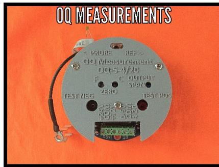
The OQ Detector Card, Model# OQ-5-4/20, comes in 0-5% BS&W with 4-20mA loop. This Detector Card is a precision replacement for the 4528 Detector and it provides superior operation when connected to the 100A Monitor and probes. The 0-5% model operates on 12 VDC only and provides a 0-5 VDC output signal, while the 4-20mA loop model requires 24 VDC. The 4-20mA loop model may be used as a 0-5 VDC output detector when connected to a 12 VDC power source.
